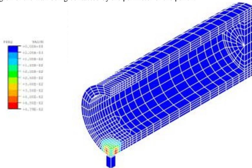
Fig. 9 Plastic strains. Perspective view
