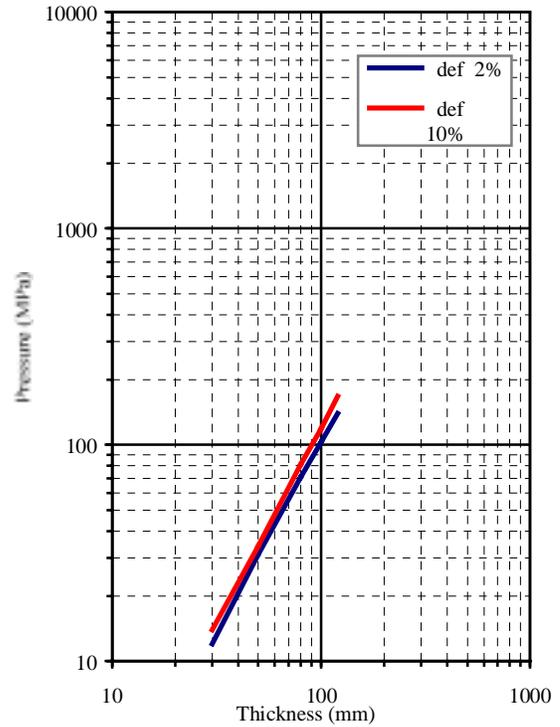
Fig. 7 Pressures inducing 2% and 10% strains
