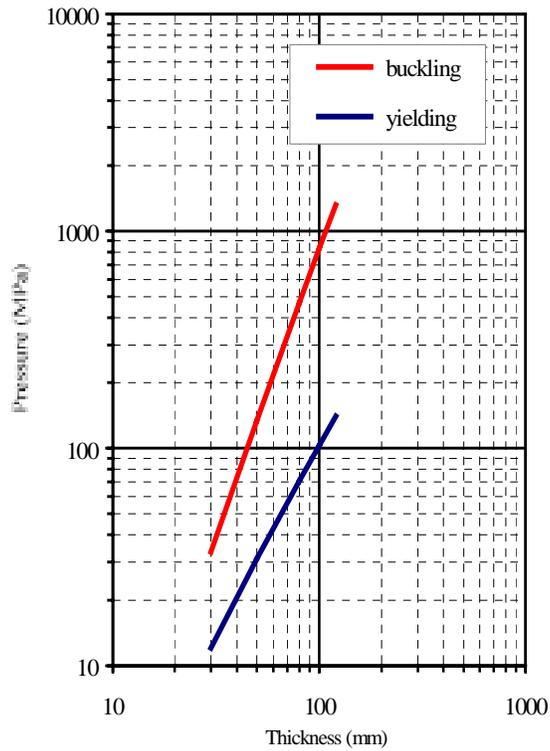
Fig. 8 Thicknesses required to avoid buckling and yielding
