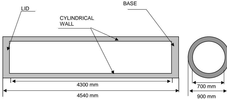
Fig. 1 General dimensions of the canister
