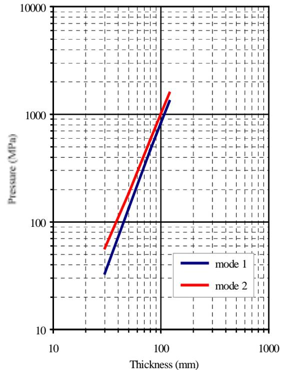
Fig. 5 Critical buckling pressure
