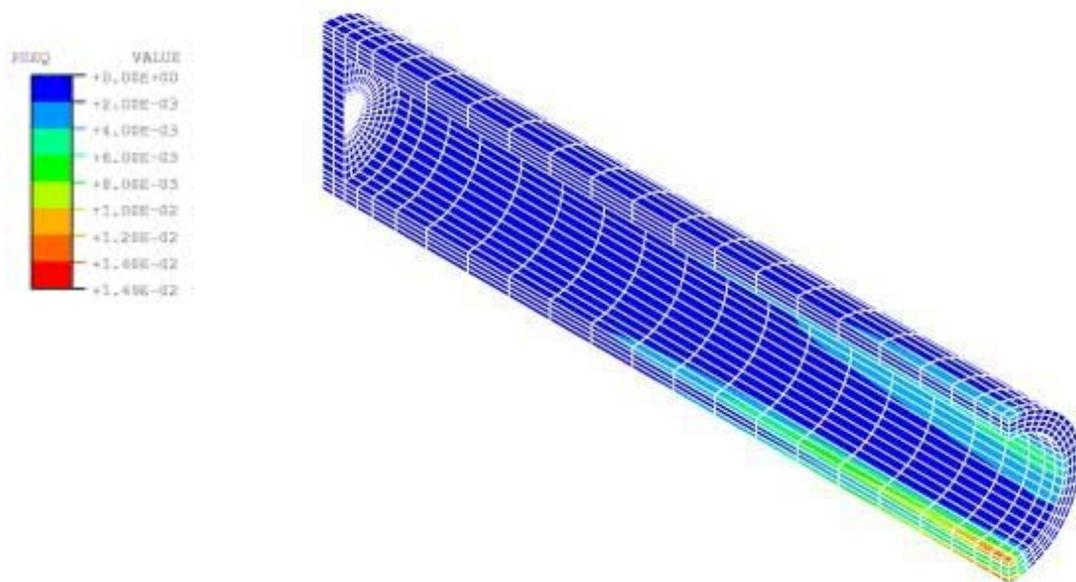
Fig. 10 Plastic strains. Perspective view
