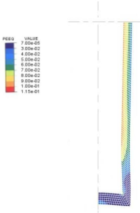
Fig. 6 Plastic strains with 120 mm wall
