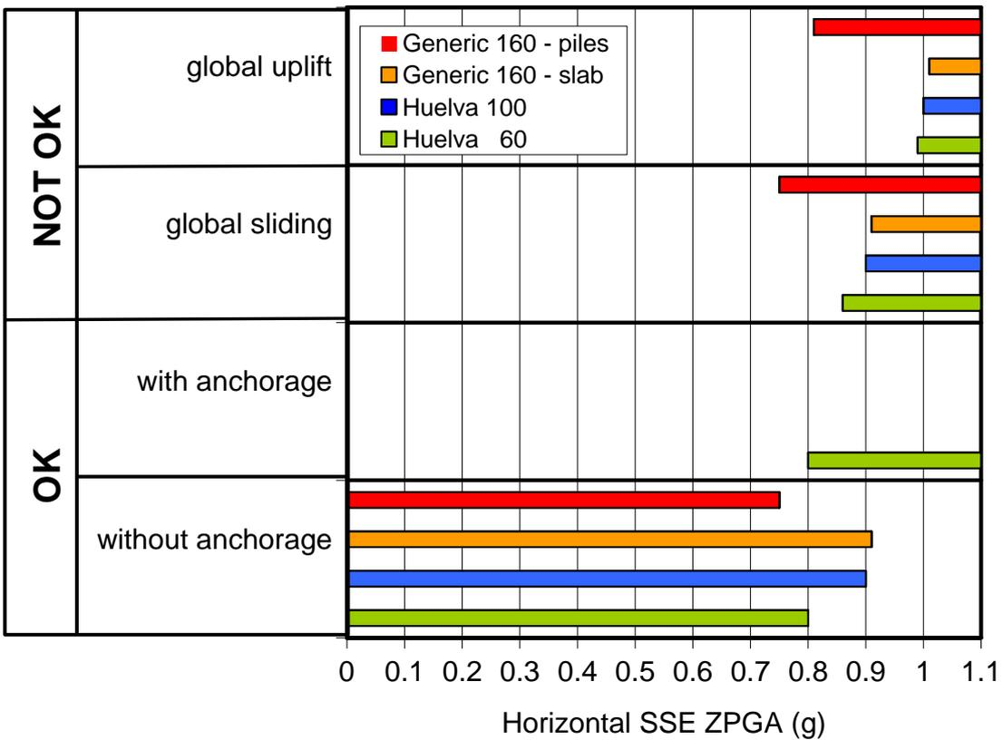
Figure 2 Onset of problems for isolated tanks. Spectrum SC
