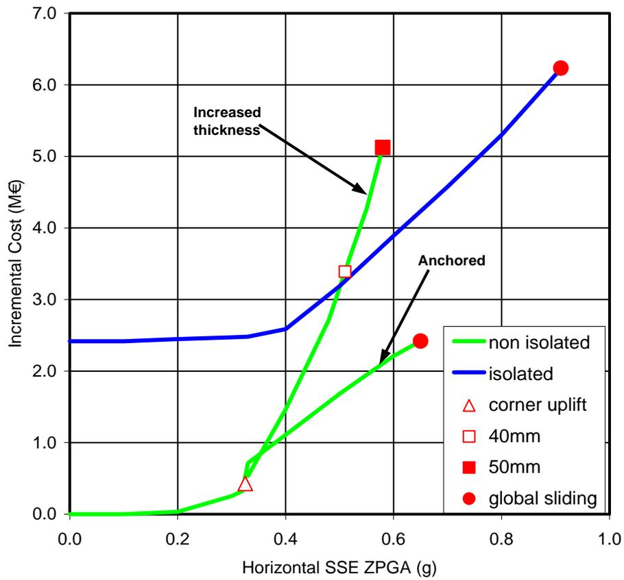
Figure 3 Cost evolution with seismic demand. Slab Foundation
