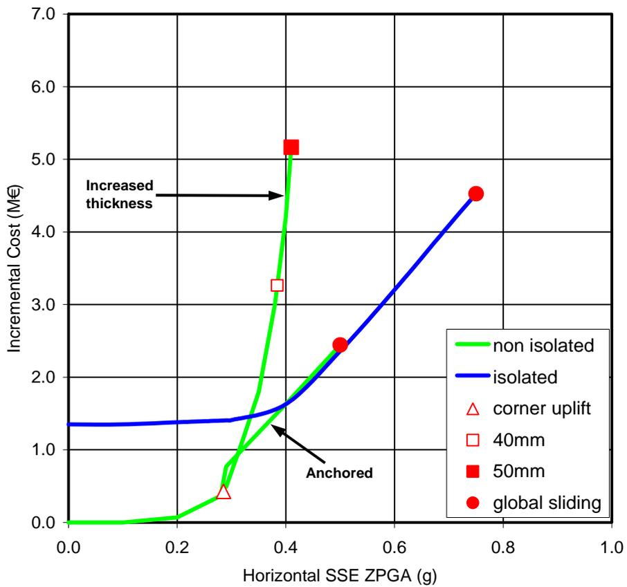
Figure 4 Cost evolution with seismic demand. Pile Foundation
