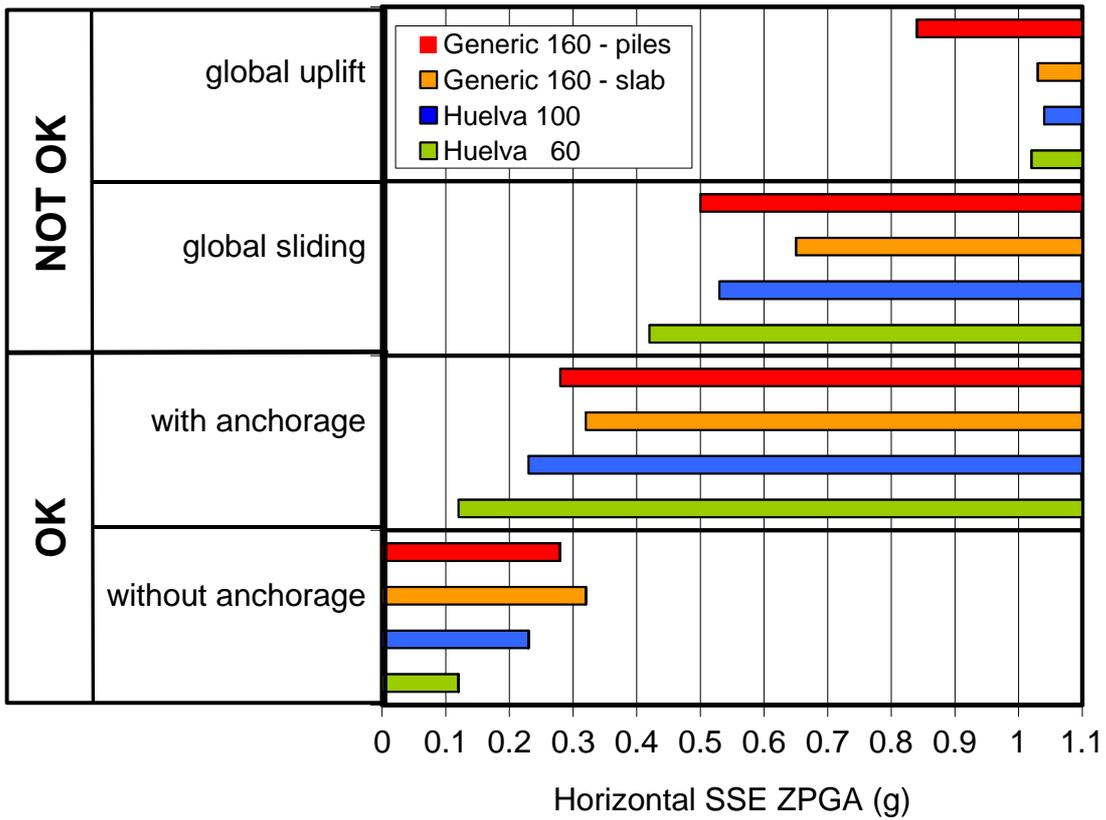
Figure 1 Onset of problems for non-isolated tanks. Spectrum SC
