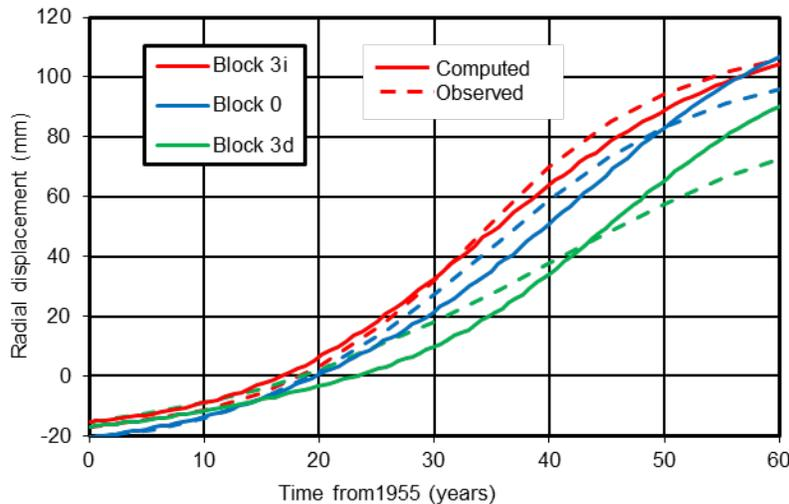
**Figure 10. Observed and computed radial displacements.**
