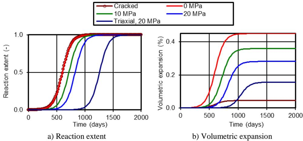
**Figure 3. Reaction extent and volumetric expansion by Saouma and Perotti (2006).**
