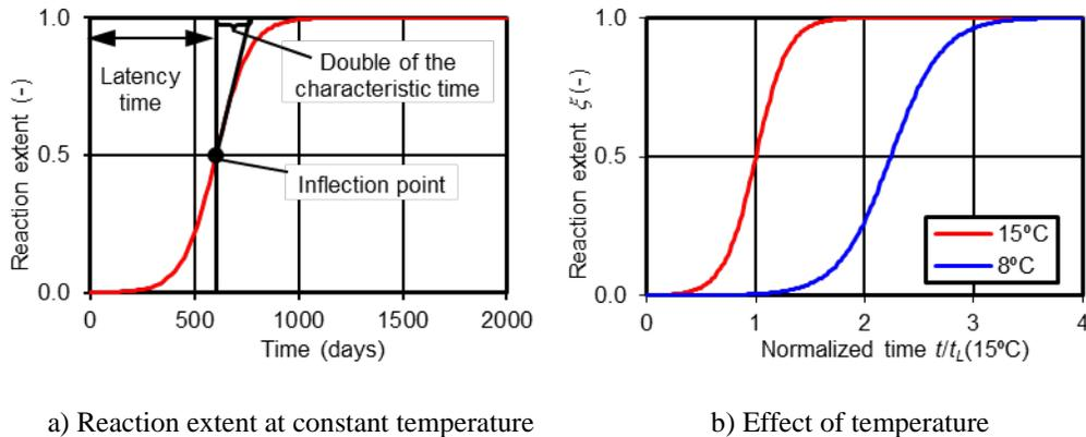
**Figure 1. Reaction extent according to Ulm et al (2000).**
