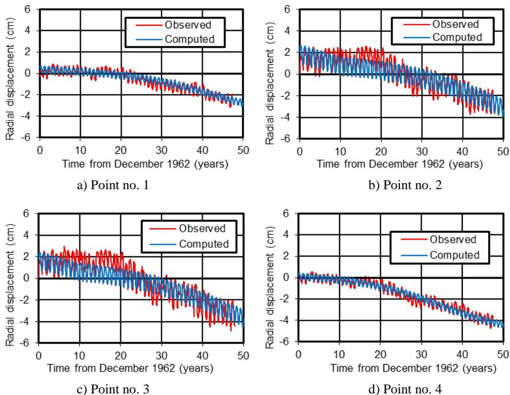
**Figure 14. Comparison of recorded and computed displacements**
