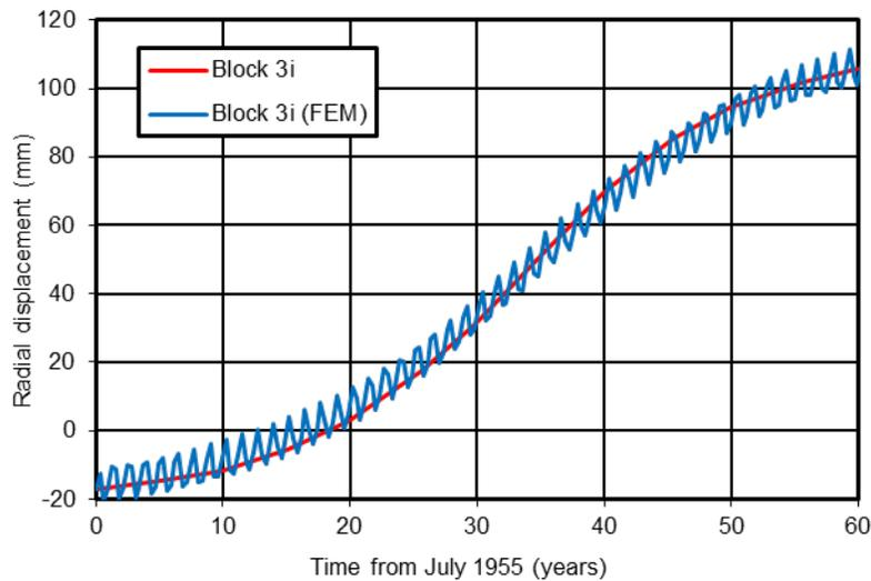
**Figure 8. Adjustment of movements in block 3i.**
