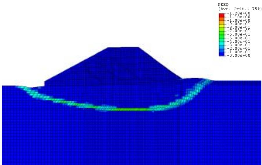
Fig. 4 Plastic strains without deterioration during construction
