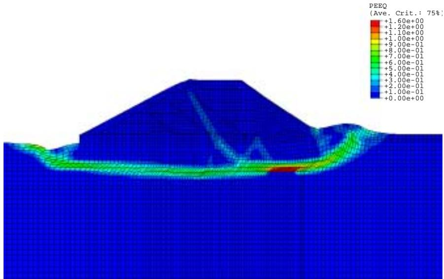
Fig. 3 Displacing dam with plastic strains
