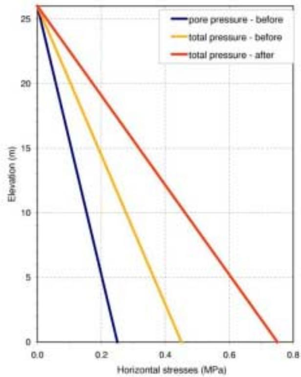
Fig. 1 Horizontal stresses before and after liquefaction
