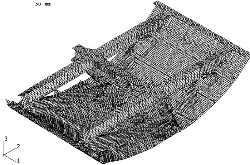
Figure 5.- Deformed mesh at 50 ms in pre-test analyses
