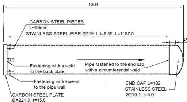
Figure 2. Drawing of the missile used in tests X3 and X4.
