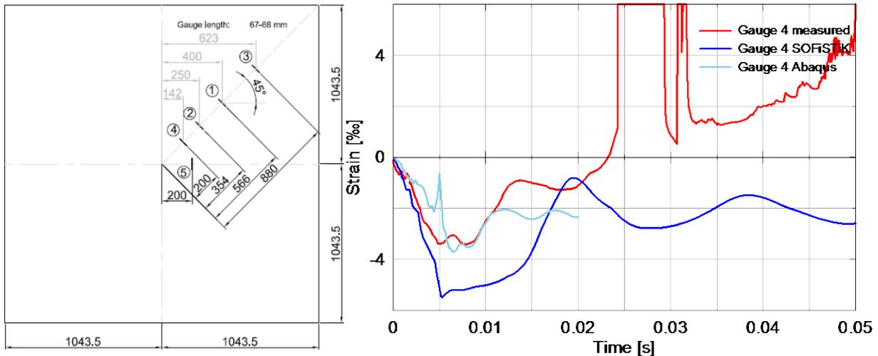
Figure 10. Comparison of concrete strains for the X3 experiment
