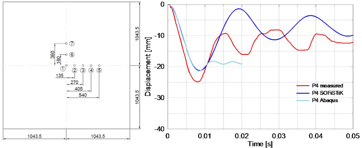
Figure 6. Comparison of displacements for the X3 experiment
