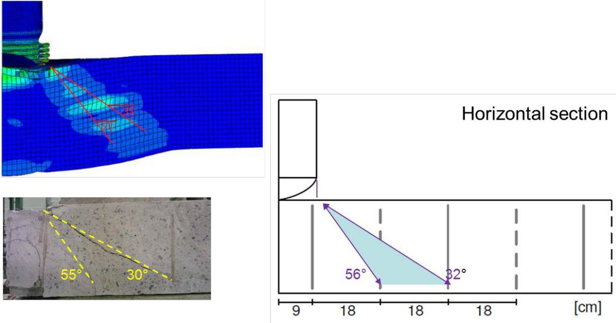
Figure 9. Computed and observed crack development related to stirrup distribution
