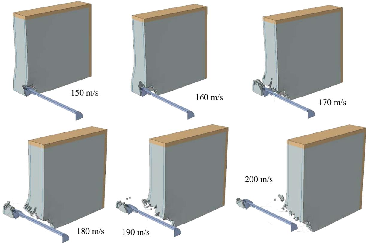
Figure 11. Deformation after 20 ms for different impact velocities
