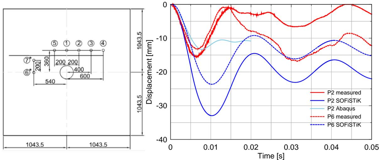
Figure 15. Comparison of displacements for the X4 experiment (front side)
