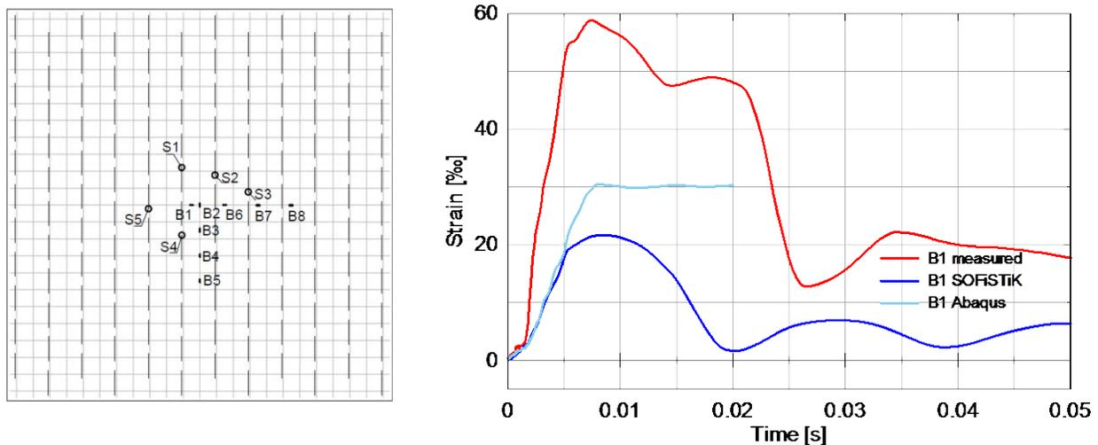
Figure 7. Comparison of reinforcing steel strains for the X3 experiment
