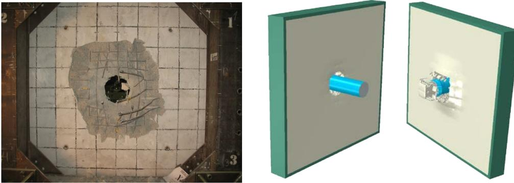
Figure 13. Rear view of plate after X4 test (photograph and FEM after 20 ms)
