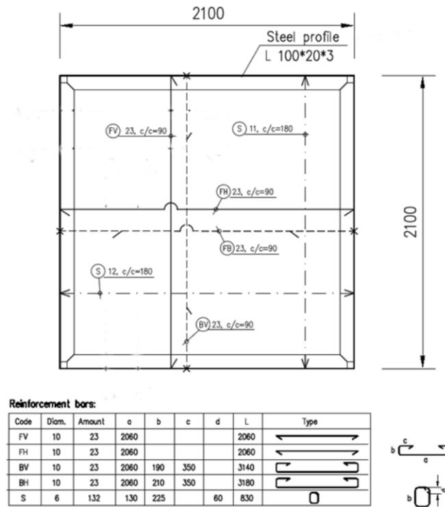
Figure 1. View of the slab and rebar quantities.
