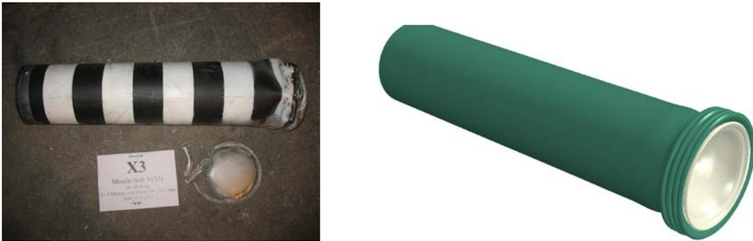
Figure 4. Deformed missile after the impact
