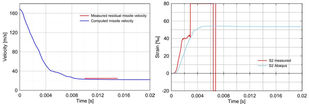
Figure 14. Residual velocity of the X4 test (left) and strains of stirrup S2 (right)
