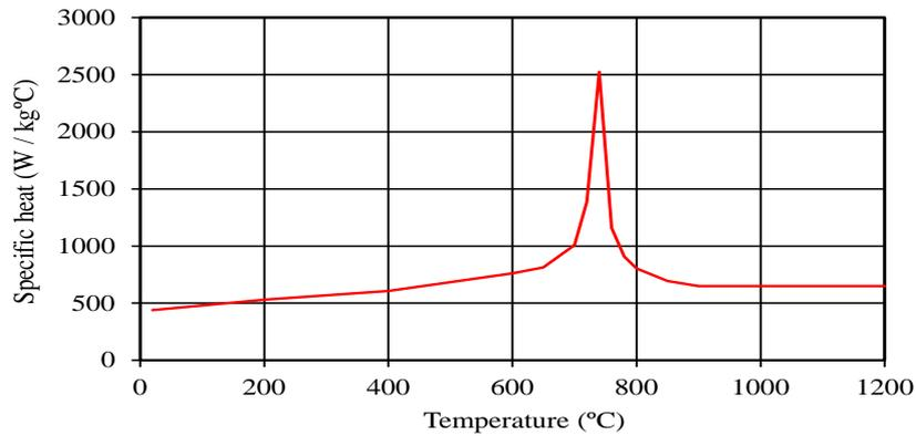
Figure 8: Dependence of the steel specific heat on temperature
