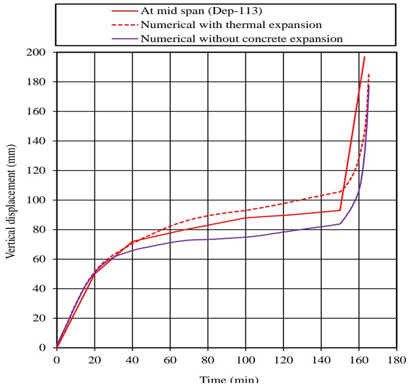
Figure 22: Comparison with and without concrete expansion
