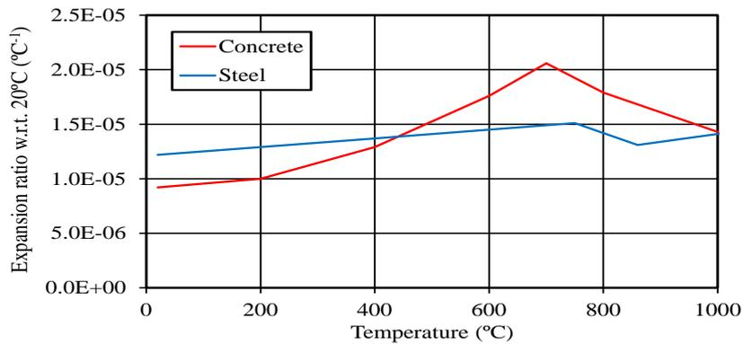
Figure 9: Comparison of the concrete and steel thermal expansion
