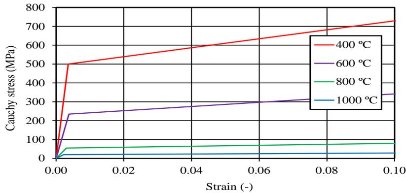
Figure 12: Rebars behaviour at different temperatures
