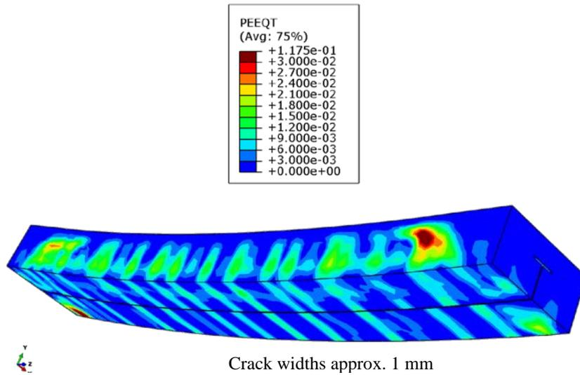
Figure 17: Equivalent cracking strains at 150 min
