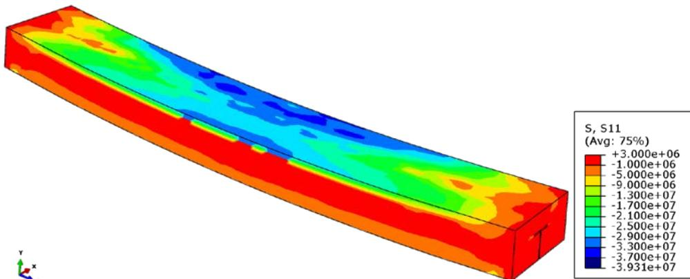
Figure 15: Longitudinal stresses in the concrete at 150 min
