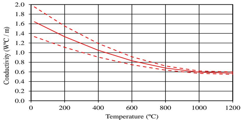
Figure 4: Dependence of the concrete conductivity on temperature
