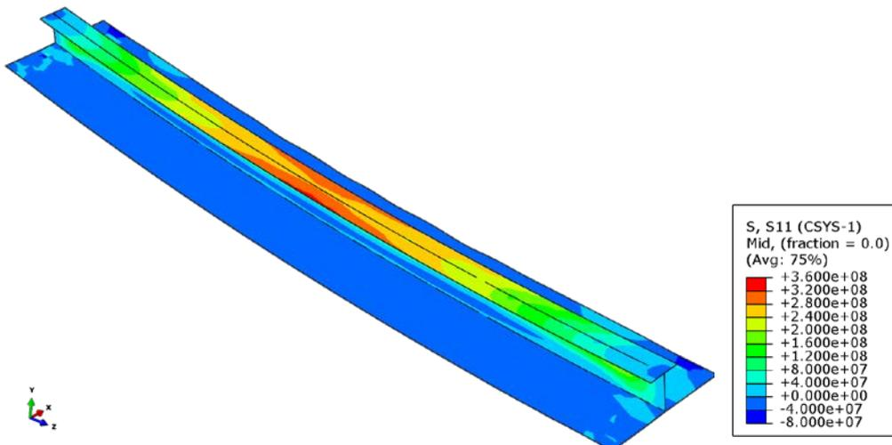
Figure 16: Long. stresses in the structural steel at 150 min
