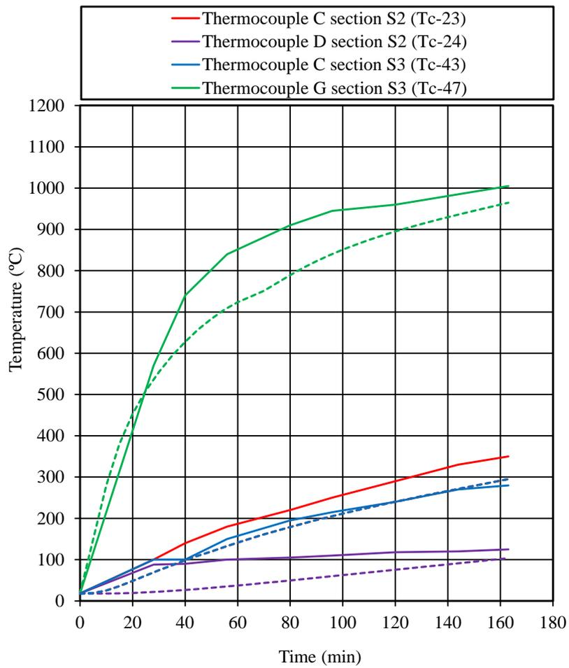
Figure 19: Comparison of temperatures in the steel plates
