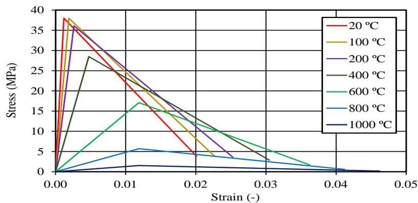
Figure 6: Concrete compressive behaviour at different temperatures
