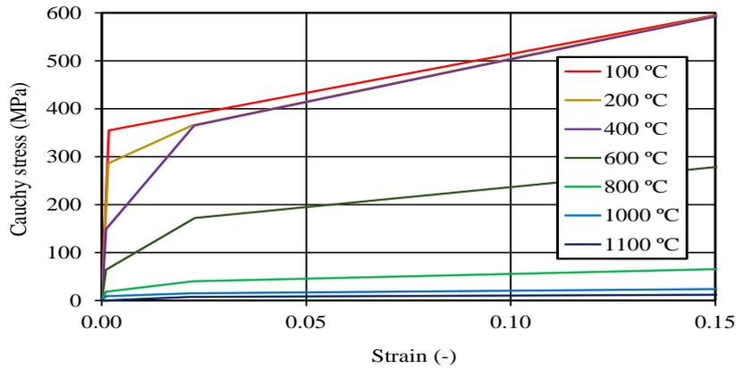
Figure 10: Structural steel behaviour at different temperatures
