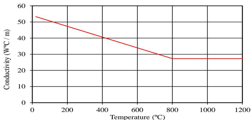
Figure 7: Dependence of the steel conductivity on temperature
