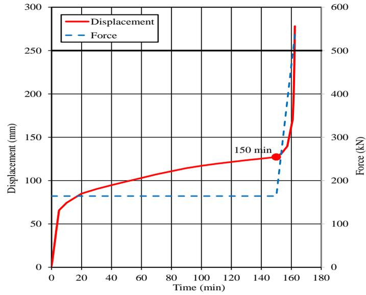
Figure 14: History of displacement at the middle of the span
