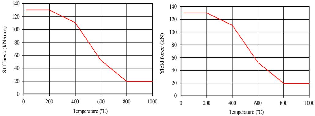
Figure 11: Dependence of the shear stud stiffness (a) and strength (b) on temperature
