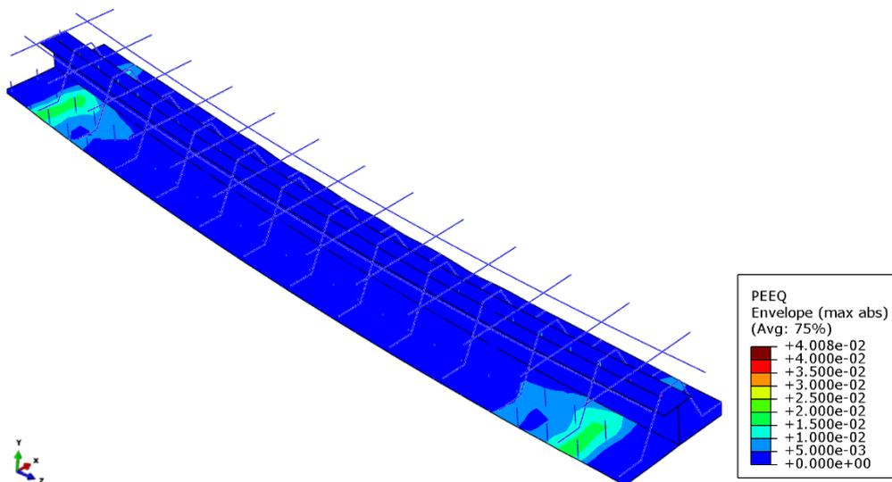
Figure 18: Plastic strains in steel and rebars at 150 min
