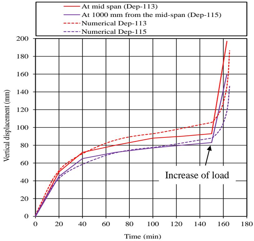
Figure 21: Comparison of vertical displacements
