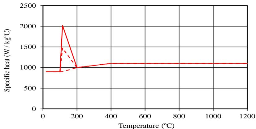
Figure 5: Dependence of the concrete specific heat on temperature
