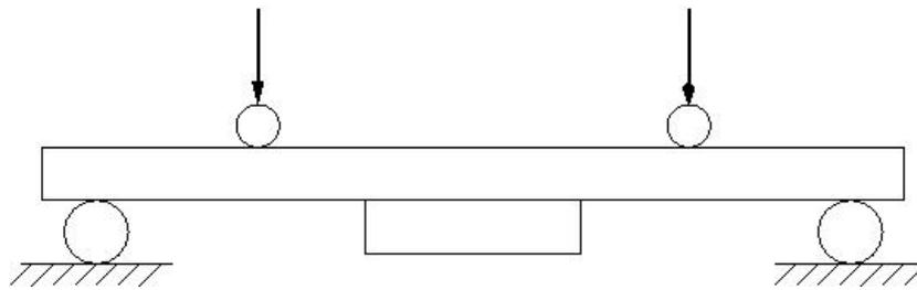
Figure 6. Configuration for 4PB test.
