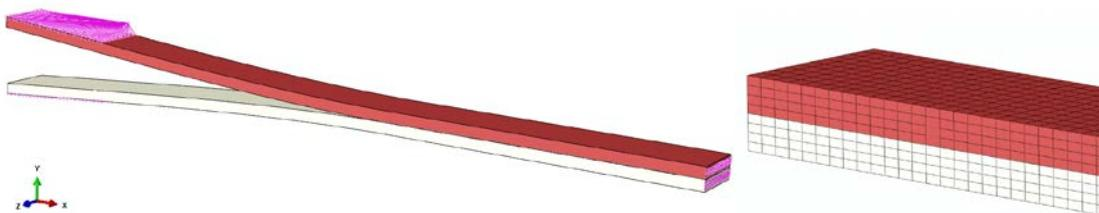
Figure 7. Finite element model for DCB test.
