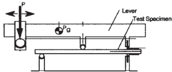
Figure 3. Configuration for MMB test.
