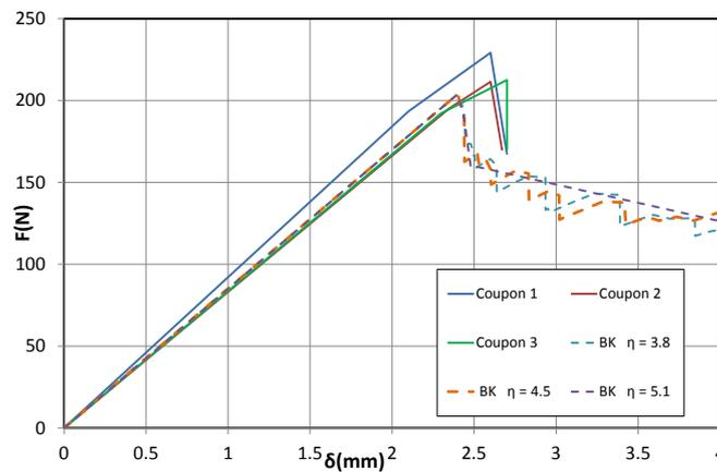
Figure 11. MMB. Force vs displacement, sensitivity to  $\eta$
