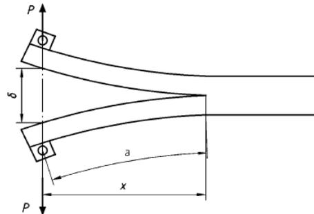
Figure 1. Configuration for DCB test.
