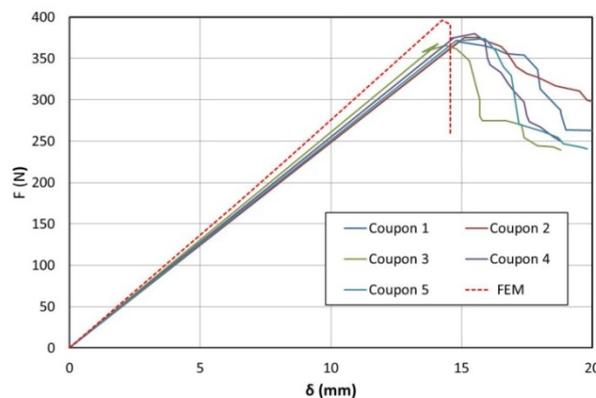
Figure 10. C-ELS test. Force vs displacement
