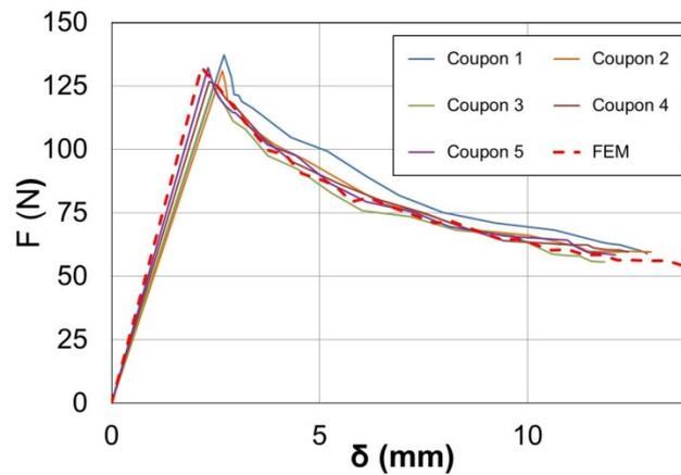
Figure 9. DCB test. Force vs displacement
