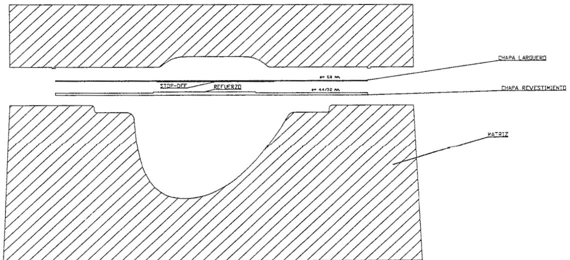
Figure 16. Simulation IV. Geometry of dies
