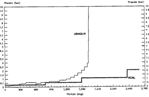
Figure 4. Simulation I. Comparison between analytical & experimental pressure cycles
