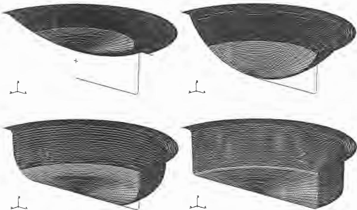
Figure 2. Simulation I. Sequence of deformed shapes in 100% top hat simulation
