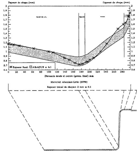
Figure 3. Simulation I. Comparison between analytical & experimental thicknesses
