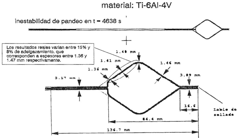
Figure 10. Simulation II. Comparison with experimental deformed shapes
