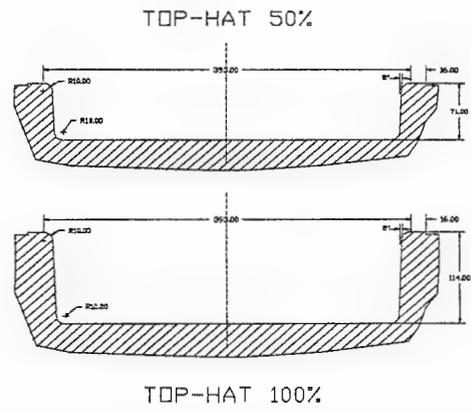
Figure 1. Simulation I. Geometry of "top hat" parts
