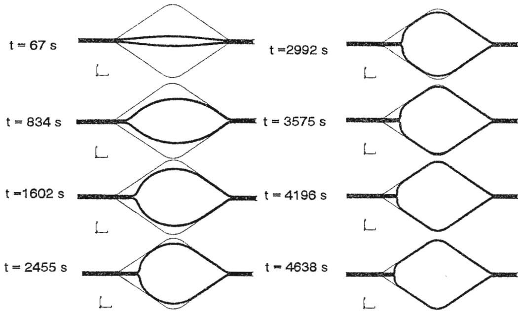
Figure 9. Simulation II. Deformed shapes in SPF simulation
