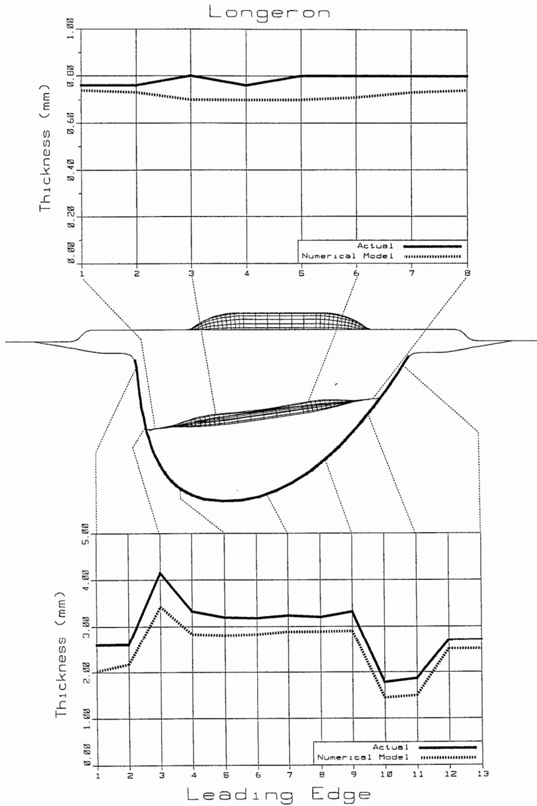
Figure 17. Simulation IV. Comparison Between analytical & experimental thicknesses
