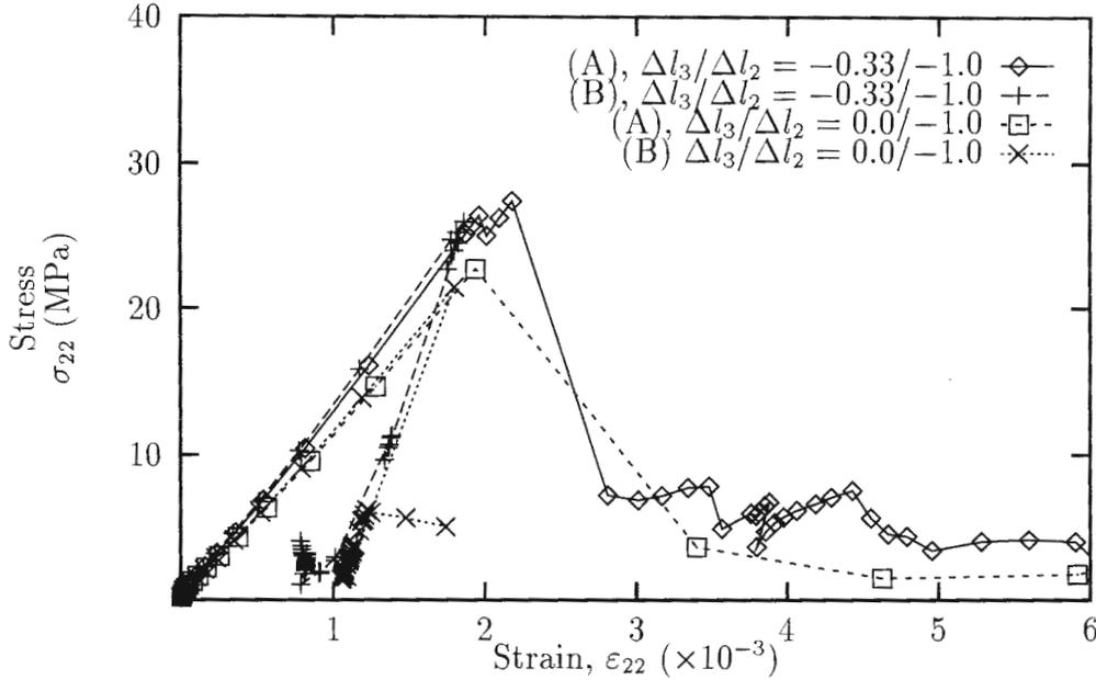
Figure 4: Axial stress vs. axial strain paths for points in two different areas within the specimen: (A) outside of fracture band, (B) within fracture band, in biaxial loading and uniaxial plane strain compression
