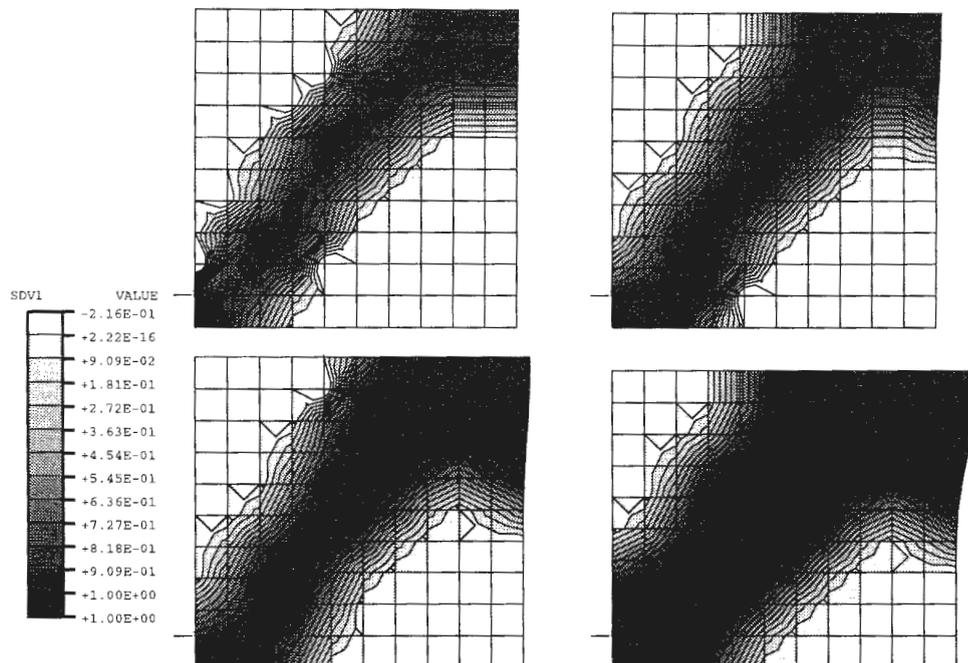
Figure 2: Sequence of deformed shapes (displacements magnified  $\times 2$ ) for the case of uniaxial plane strain compression ( $\Delta l_3/\Delta l_2 = 0.0/-1.0$ ). The fringe levels indicate the cracking process in the mortar, indicative of the evolution of the localised shear band.
