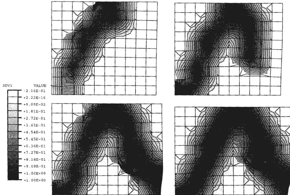
Figure 1: Sequence of deformed shapes (displacements magnified  $\times 25$ ) for the case of biaxial loading ( $\Delta l_3/\Delta l_2 = -0.33/-1.0$ ). The fringe levels indicate the cracking process in the mortar, indicative of the evolution of the localised shear band.
