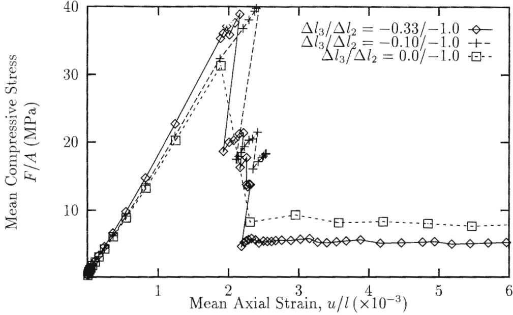
Figure 3: Mean axial stress vs. mean axial strain curves for two different biaxial load paths and uniaxial plane strain compression
