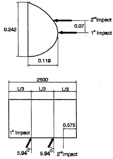
Figure 2. Test set up.
