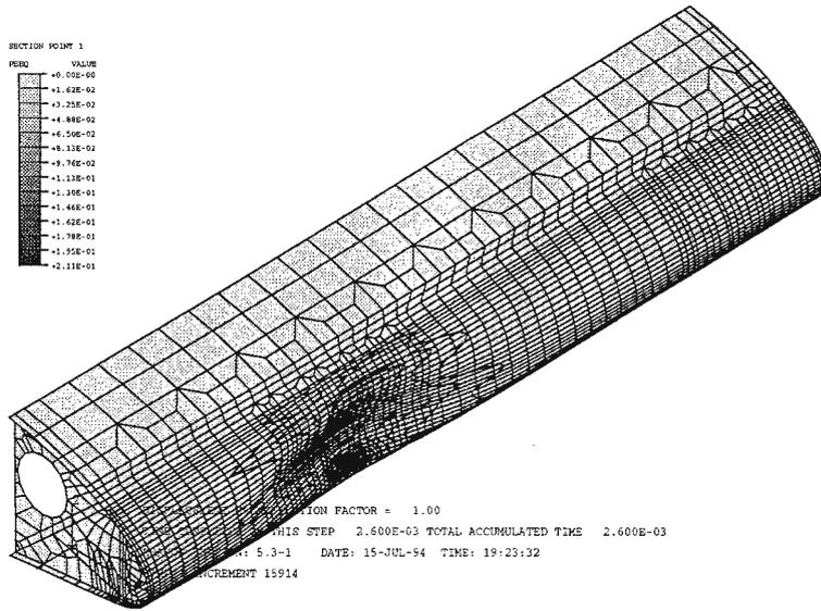
Figure 6. Contours of effective plastic strain at 2.6 ms.
