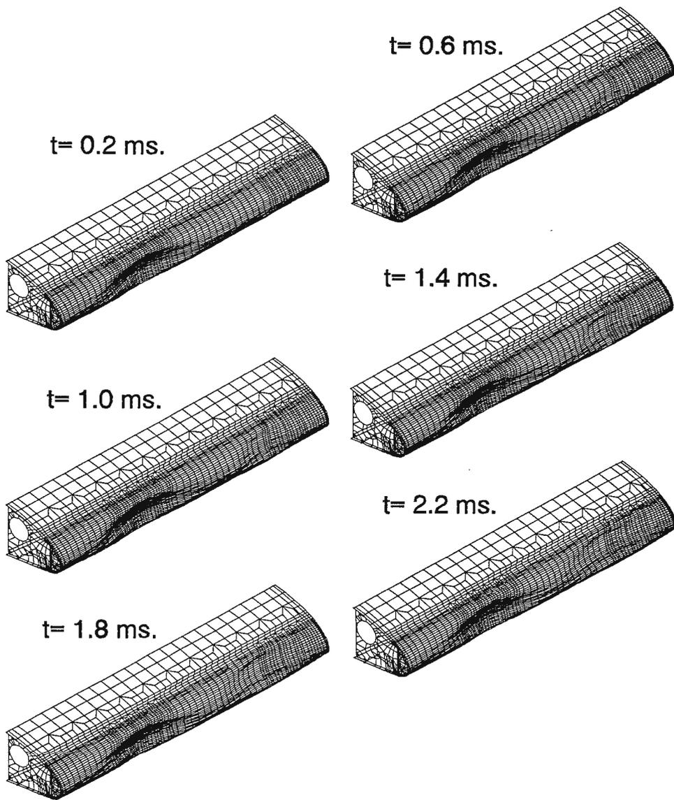
Figure 9. Sequence of deformed configurations.
