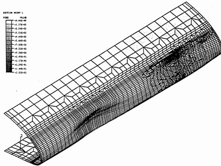
Figure 10. Contours of effective plastic strain at 2.2 ms.
