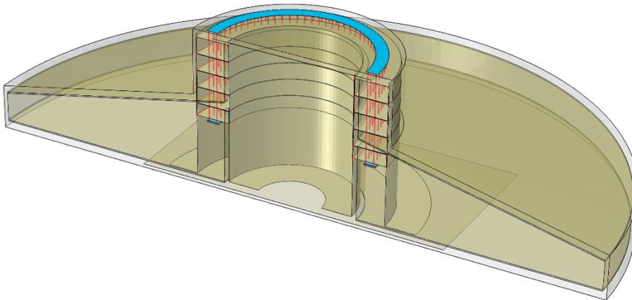
**Figure 4. Geometry of a foundation with post-tensioned bolts.**
