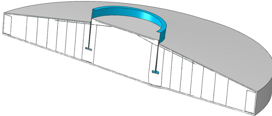
**Figure 8. Deformation at failure point (deformation scale x20).**
