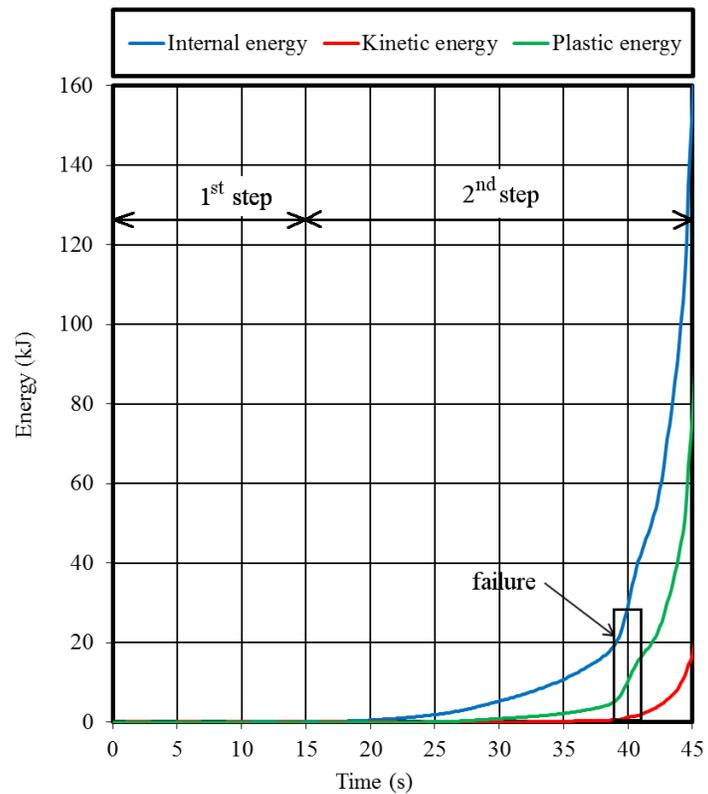
**Figure 7. Evolution of energies during the loading process.**
