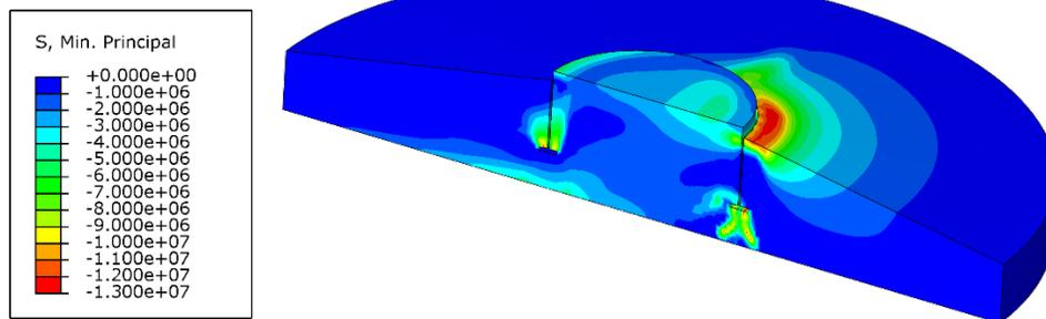
**Figure 9. Compression in concrete (Pa).**
